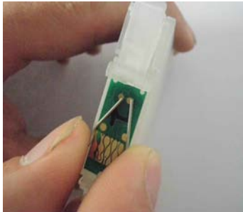
4. using wire to connect 2 point show on picture (2-3 seconds)
