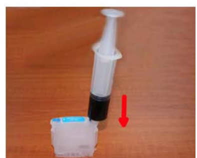
6. Please make them join well, or the Ink will leak during filling. It will also leak air.
