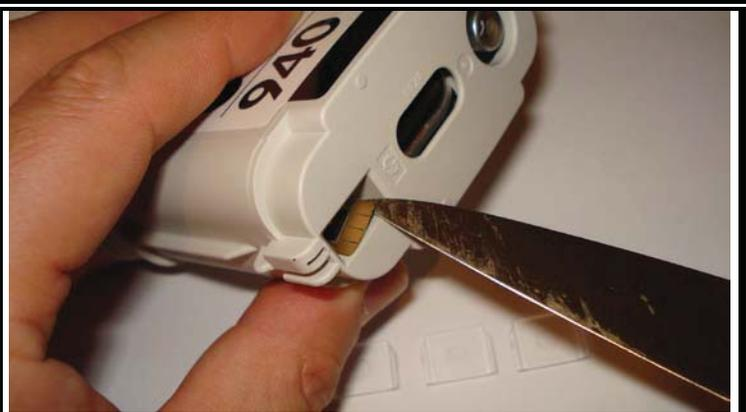
With a thin knife, gently slide the blade underneath the chip on the original cartridge and slowly, carefully, rock it back and forth until you have small gap between the chip and cartridge. Continue moving the blade to release any of the glue that is on the back of the chip until the chip releases from the cartridge.
