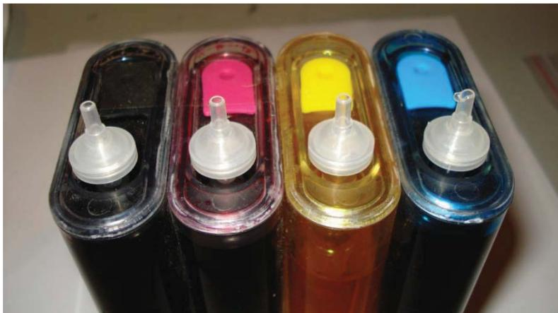
Take the air plug off, which is the smaller plug on the top of the ink tank, then put the air filter down. The air filter has two sides, just put the thicker side down.
