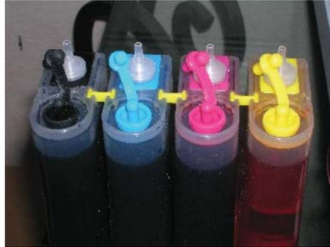
Pull out the small rubber plug from the air holes on the ink tanks and insert air vents as pictured above. If you do not install these air vents, you will create a vacuum in the lines and your printer will not print after about three pages.
