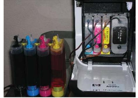
Install your cartridges with lines going to the left as pictured above and ink tanks placed on the same level surface or up to 6" above your printer. If needed, gently separate the ink lines to give you room to feed them out to the left. Make sure that you press each one in firmly starting with black and moving over to the left.
