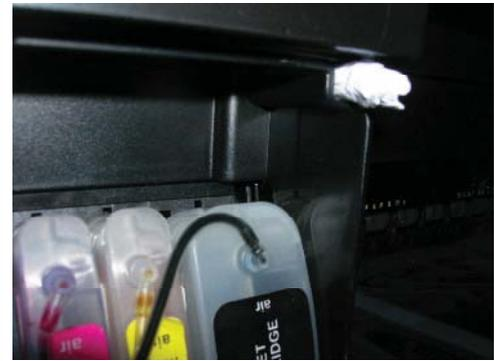
**Optional Step:** If you are concerned about the ink lines possibly being crimped, you may leave the cartridge door open, just twist up a small piece of paper and insert into the cartridge door sensor. This will allow you to print with the door open with no risk of crimping lines.
