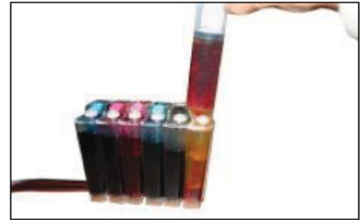
Please pay attention to the ink level in the reservoirs; if the ink level is below 1CM as the picture shown above, please use refill kits to fill ink into Reservoir bottles. Carefully pull out the rubber plugs from the ink refill holes (There is possibility of ink spattering. Please be careful.) Refill ink according to the colors. Then re-cap the rubber plug. **(Please keep the printer and the reservoir bottles at the same level while refilling ink.)**
