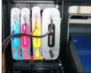
Open cover for Inkjet cartridges remove the original cartridges Insert our no-sponge cartridge into printer carefully
