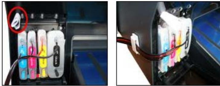
Use paper make taper style and Finished Insert the paper into the printer hole .Then cartridge-cover can be recognized cover well.
